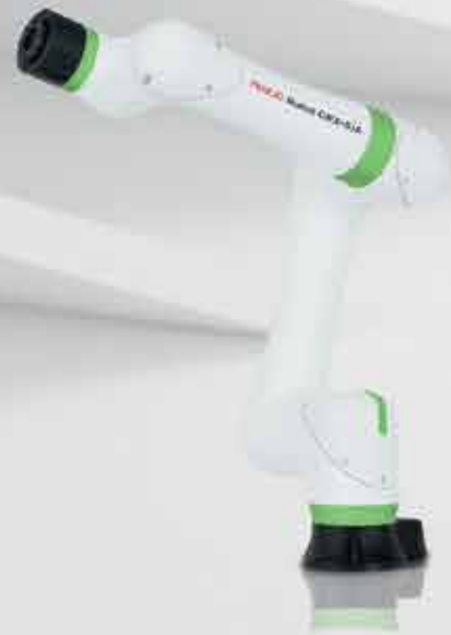
CRX-5iA Payload: 5 kg Reach: 994 mm
