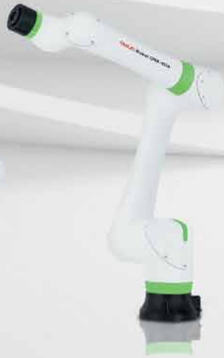
CRX-10iA Payload: 10 kg Reach: 1,249 mm
