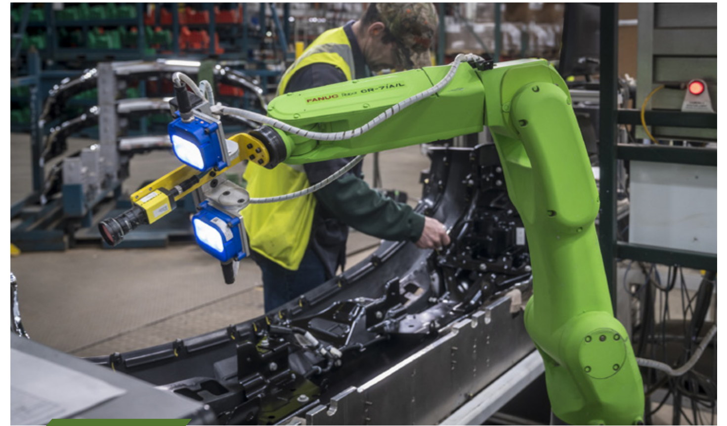
↑ A Fanuc CR-7iA/L robot equipped with machine vision technology inspects car bumpers for defects working alongside an operator.
