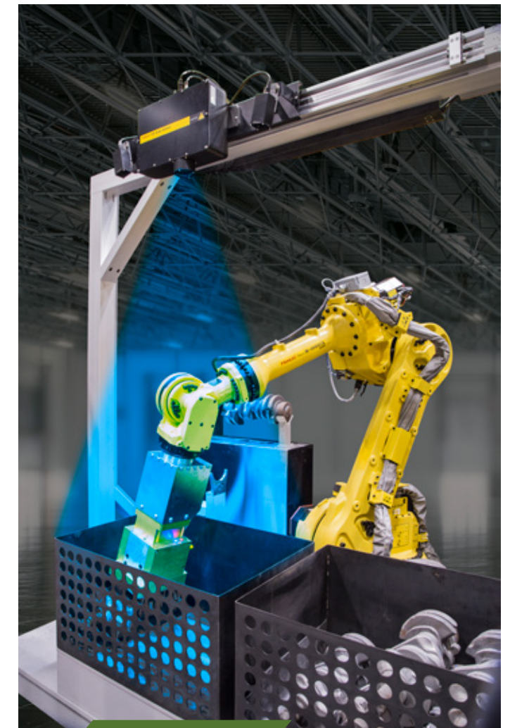
↑ Fanuc's R-1000iA robot uses iR-Vision's 3-D Area Sensor for bin picking parts.
